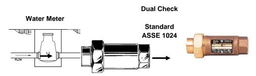
**Description** (**DuC**). A dual check shall contain two internally loaded, independently operating check valves. A dual check shall be a device approved by an approval agency acceptable to the local administrative authority.
